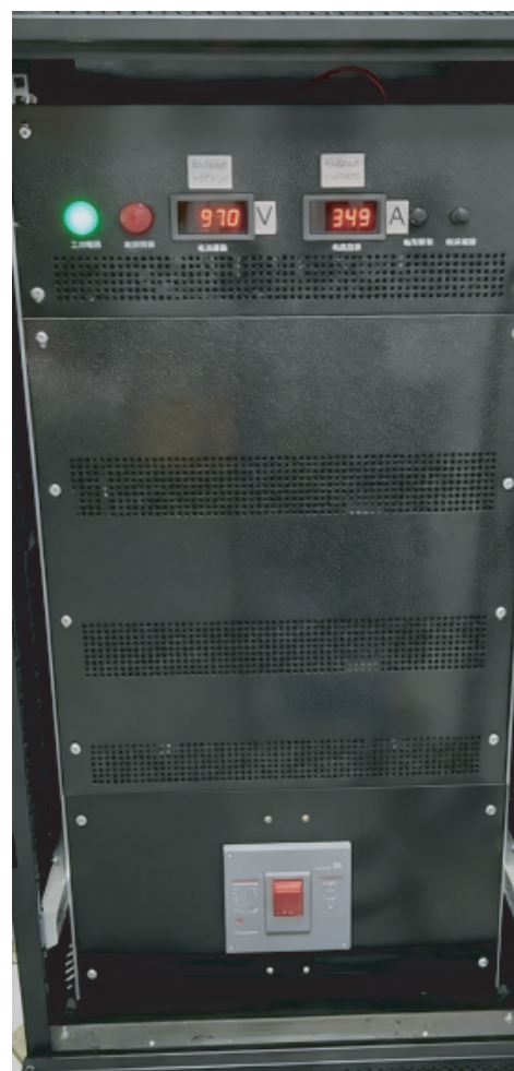
Figure 4-2 Image of DC Power Supply
